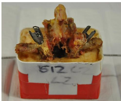
**Figure 2** Example specimen potted in polymethyl methacrylate (PMMA) and instrumented with minimally invasive surgical (MIS) and open techniques on opposing sides. In this specimen, the open insertion site is seen on the left and the MIS on the right. The techniques were alternated for adjacent vertebrae.
