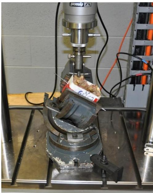
**Figure 5** Test setup, showing specimen clamped in vice which is fixed to the Instron base. The linear actuator is coaxially aligned with the axis of the screw for the pullout test.
